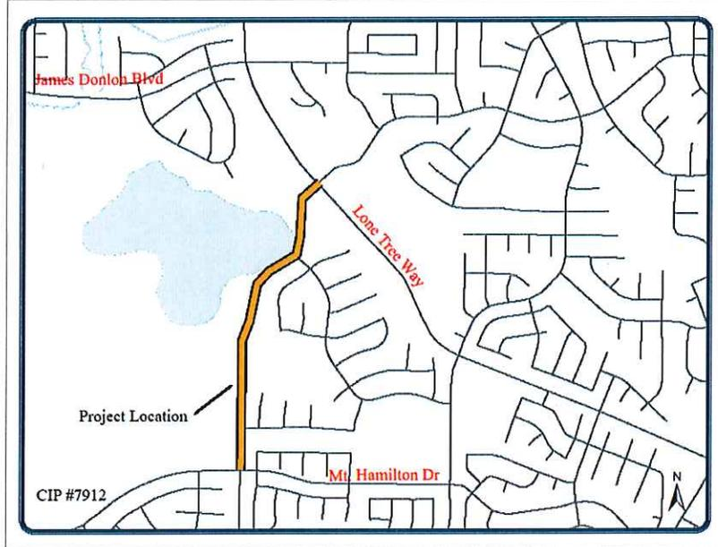
**Project Description:** The project will identify and replace curb, gutter and sidewalks that have been damaged or raised due to tree roots and remove existing trees. The damaged pavement area will be resurfaced with the Pavement Rehab Program Project.
