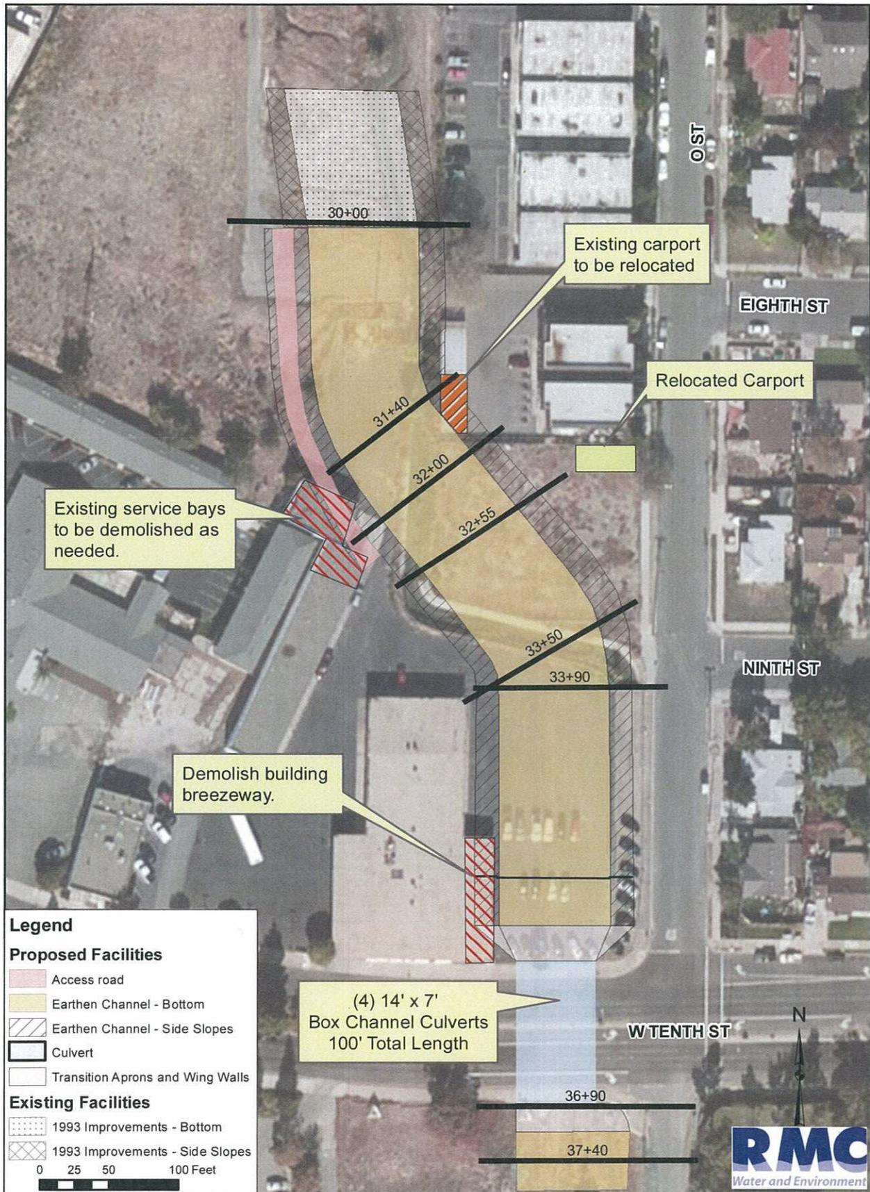
Figure 1. Alternative 3A: Revised Alternative Minimum Culvert Option
